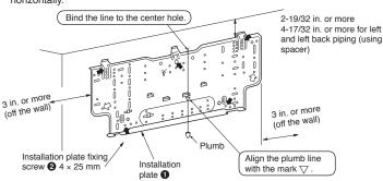
To prevent the installation plate from vibrating, be sure to fix the holes as indicated by the arrows 1.
