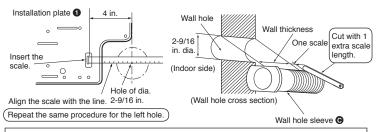
Be sure to use wall hole sleeve ( to prevent the outdoor connecting wires from contacting with metal part in the wall and to prevent damage by rat in case the wall
