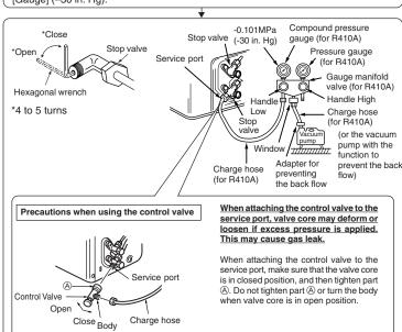
Remove the gauge manifold valve quickly from the service port of the stop valve.
