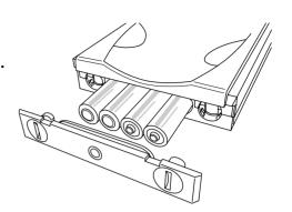
5. Insert the battery cover, and tighten the locks on the cover. Ensure that the wireless controller display lights up and that the battery life indicator is fully lit.
